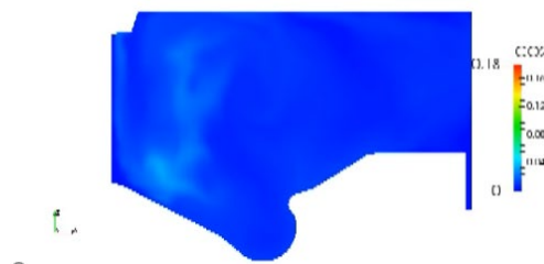
Figure.3 CFD visualization of CO 2 fraction in the engine combustion chamber during the power stroke at 40
